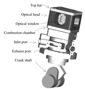
Fig. 2. CAD drawing of the Proteus Engine
