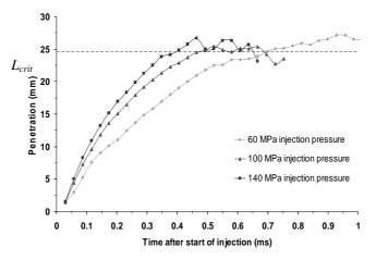
Fig. 9. Effect of injection pressure on spray penetration for a 0.135 mm 7-hole single guided VCO nozzle, at 6 MPa incylinder pressure and cold air intake, showing the definition of  $L_{crit}$
