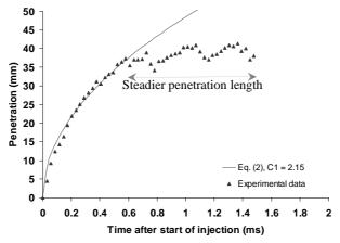
**Fig. 12.** Comparison between empirical constants and experimental data; the experimental results are for non-evaporating spray (cold intake); 160 MPa injection pressure; 4 MPa ICP, 24.2 kg m<sup>-3</sup> ambient gas density
