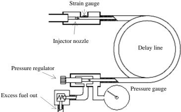
Fig. 1. Schematic diagram of Lucas rate tube
