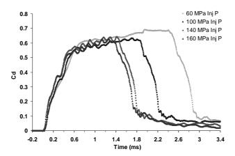
Fig. 4.  $C_d$  as a function of time, for a 0.2 mm single guided 3 hole VCO nozzle at 4 MPa back pressure, and 50 mm<sup>3</sup> fuelling
