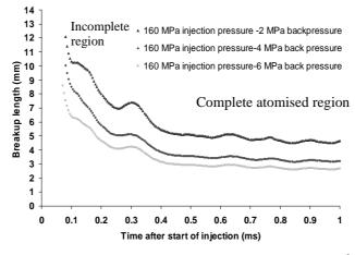
**Fig. 13**. Maximum breakup length  $(L_b)$  as a function of time from start of injection, and 50 mm<sup>3</sup> fuelling
