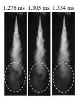
Fig. 6. High-speed video sequence in steps of 29 μs showing droplet clusters starting to detach along the leading edge of the spray at cold intake
