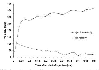
**Fig.7** Evolution of injection velocity obtained from the rate measurements, and the tip velocity obtained by differentiation of the penetration data; injection pressure 140 MPa; in-cylinder pressure 6 MPa cold air intake; 0.135 mm VCO single guided 7 hole nozzle
