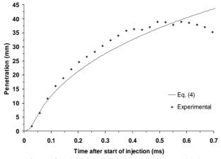
**Fig.11** Calculated position of centre-of-mass for the injected fuel and experimentally observed spray tip for a 0.135 mm 7-hole single guided VCO nozzle, at 140 MPa injection pressure and 2 MPa in-cylinder pressure at TDC; cold intake. The model parameters are  $Re_{initial} = 0.831$ ,  $C_{blasius} = I$ . Experimental value for  $L_{crit} = 37.5mm$
