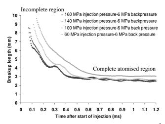
Fig. 14. Maximum breakup length  $(L_b)$  as a function of time from start of injection, and 50 mm<sup>3</sup> fuelling
