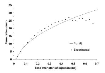
**Fig.10** Calculated position of centre-of-mass for the injected fuel and experimentally observed spray tip penetration for a 0.135 mm diameter 7-hole single guided VCO nozzle, at 140 MPa injection pressure and 6 MPa in-cylinder pressure at TDC; cold intake. The model parameters are  $Re_{initial} = 0.831$ ,  $C_{blasius} = 50$ . Experimental value of cluster-shedding length  $L_{crit} = 24.5mm$  can be assessed from the in Fig 9
